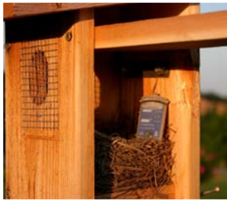
Figure 3. HOBO Pendant hourly temperature data logger inside the bluebird nest box.
